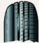
Feathered Wear (excessive toe in or out)
