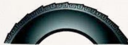
Diagonal Wear/Heel and Toe Wear
