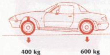
Weight transfer to rear during acceleration.
